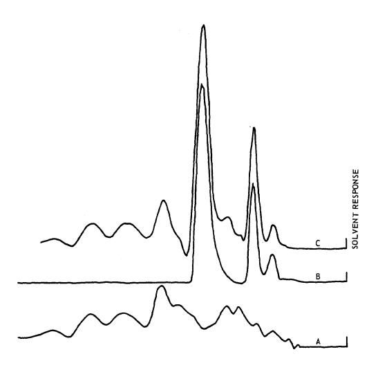
ELECTRON CAPTURE DETECTOR RESPONSES TO: A -7 NANOGRAMS TOXAPHENE, B -2.8 NANOGRAMS DDT, C -7 NANOGRAMS TOXAPHENE + 3.5 NANOGRAMS DDT
